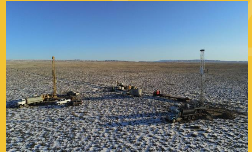
MUD ROTARY DRILL RIGS OPERATING AT THE THOR PROJECT, GDB, WYOMING
